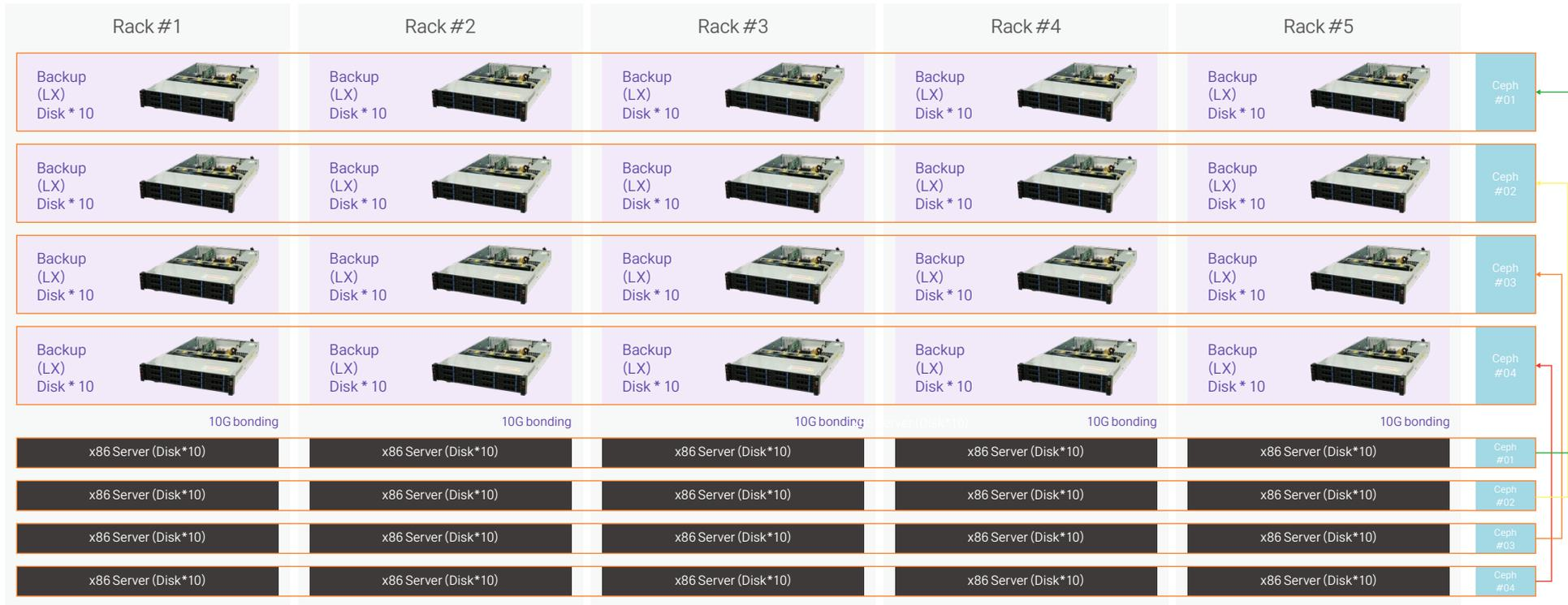
We delivered and built a V-Raptor LX server with 50 disks configured as Ceph in the same environment as the existing environment for data backup of the existing x86 server in use at KATECH.
